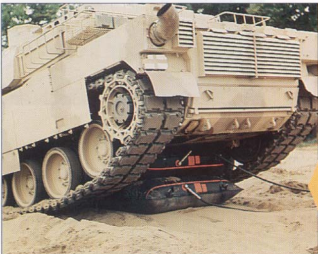
Recovery Air Lifting Bags 920 x 920 mm acting as stabilizers.
