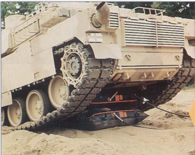
Recovery Air Lifting Bags 920 x 920 mm acting as stabilizers.
