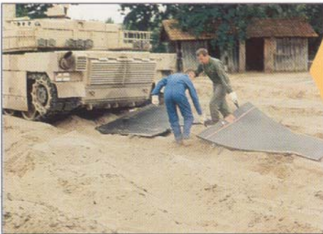
Two Recovery Air Lifting Bags 2000 x 1800 mm are easily slid under the armoured vehicle.
