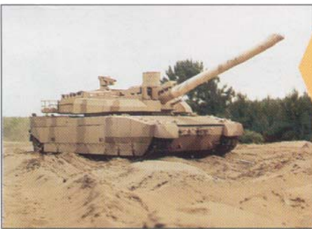
Armoured vehicle trapped in sand. Hull in contact with sand.
