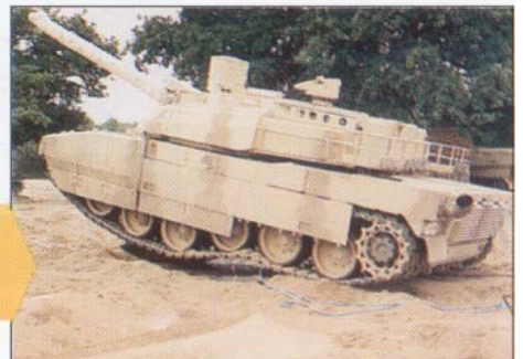
Lifting with two Bags 2000 x 1800 mm inflated at 2,5 bar with a compressor
