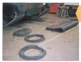
One deflated 2000 x 1800 mm Lifting Bag under the armoured vehicle. The other folded Lifting Bag is ready to be installed.
